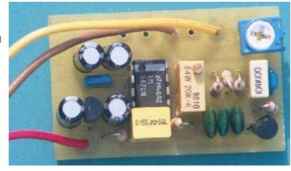
A simple CTCSS encoder (See Circuit Fig 2) was described by Will McGhie's Repeater Link column in July 1996 AR (page 46) and this article should be referred to for a full description of the encoder operation. It is based on a NE567 tone decoder IC which has either a square wave or triangle wave output from its oscillator. The triangle output is used and passed through a three stage RC filter which gives a near sine wave output. This is then buffered and fed to the output.
